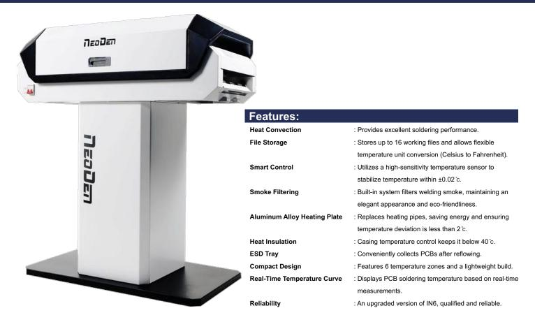
The IN6C, a newly designed and manufactured reflow oven by NeoDen Tech, boasts six temperature zones, a built-in welding smoke filtering system, working file memory function, and a heat-up reminder. These features contribute to its intelligence, innovation, and compact design.
